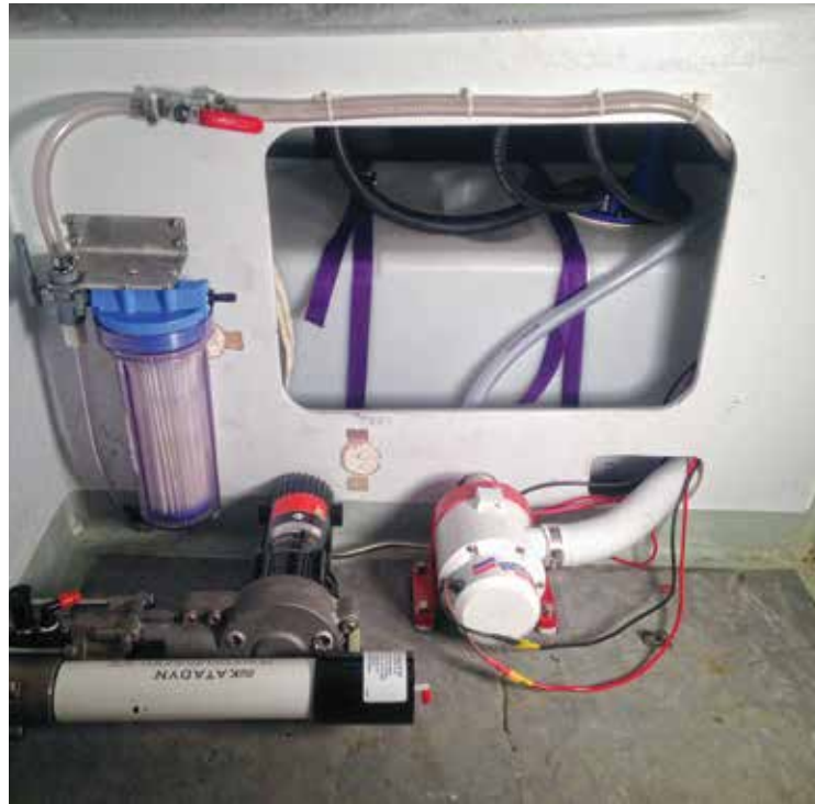
Plentiful fresh water is a necessity for every offshore sailor, including solo ones. With that in mind, I replaced my old water tank with a new 12-gallon tank, and installed a Katadyn watermaker as well (left). This tank may seem small for most cruisers, but was based on the premise that it will be replenished daily. My carbon-fiber rig was also given a complete overhaul (right). The mast was unstepped, all its hardware and rod rigging were removed and either replaced or serviced, and then it was painted with a flat-black paint with plenty of UV protection.
